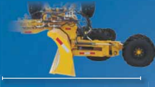
Blade angle adjustment - horizontal (from 15 to 30 degrees)
