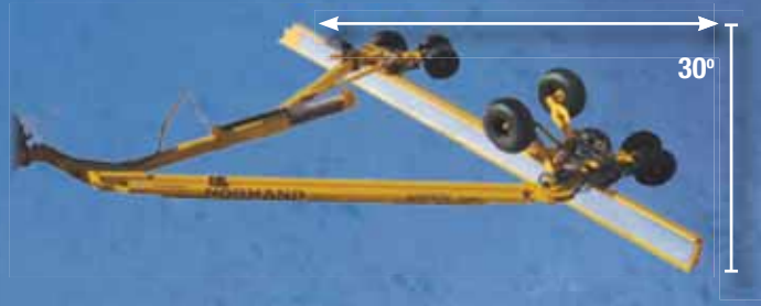
Blade angle adjustment - horizontal (from 15 to 30 degrees)
