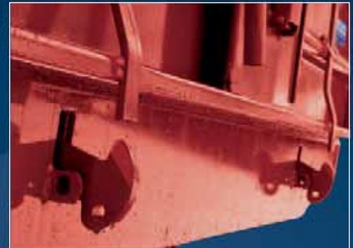
Automatic opening and closing mechanism in the rear panel.
