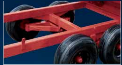
Tandem axle : Decentralized walking beam distributes more weight on the back wheels and reduces wheel skidding in sharp turns.
